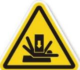
Mechanical and hydraulic lifting devices can tip over or lower accidentally due to incorrect maneuvering or technical errors. A falling object can cause injury and/or loss of life to yourself and/or others. When working under the vehicle, always use stands, and ensure that the ground or floor is stable and level. Never crawl under a vehicle which is only supported by a jack.
