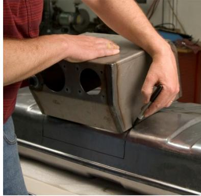
1-7. Using an appropriate saw, cut the bottom of the fuel tank to accept the sump. It is usually best to cut the hole a little small to start with. Then gradually enlarge the hole until the sump edges just fit inside of the hole.
