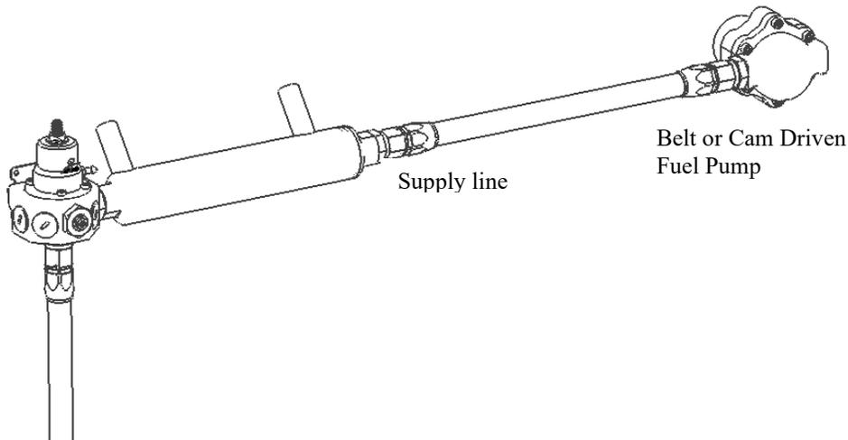
5. Attach the fuel supply line to one of the AN-08 ports located around the perimeter of the regulator using AN-8 style fittings and o-rings.
