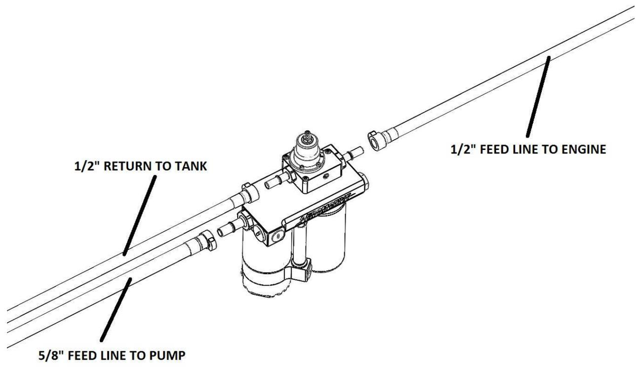
1. Select and install the pressure spring that best fits your pressure range. To swap springs, simply remove the four socket head cap screws, remove the top cap and replace spring. **FIGURE 1-1**
