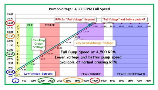
IMPORTANT: The FPSC is not a voltage booster, though theoretically one could be used in conjunction with the FPSC (done by connecting the output from a voltage booster to the FPSCs BAT terminal), maximum voltage output from the FPSC can never be more than the voltage input. Maximum voltage input should not exceed 20-volts and current draw is limited to 30-amps continuous.
