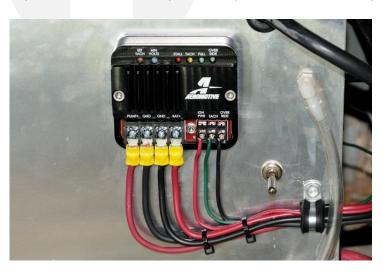
Important: The MIN VOLTS setting (the slowest fuel pump speed possible) must be set correctly for the FPSC to operate the pump properly across the engine's RPM range. The 16306 Fuel Pump Speed Controller ties fuel pump speed to engine RPM, speeding the pump up and down with the engine.
