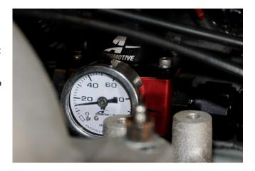
7.) If the fuel pressure is the same with the manual override off as it is on, reduce pump speed by turning the adjusting screw counter clockwise, until the fuel pressure droops. Do not allow the pressure to droop more than 1-2 PSI from full speed base pressure. If necessary, turn the adjustment pot back in the clockwise direction to minimize pressure droop. Fine tuning the MIN VOLTS setting for the lowest speed that maintains desired base pressure allows the FPSC to be most effective.
