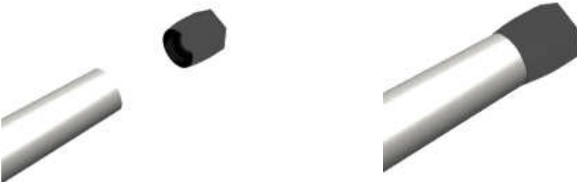
2-4. Using a grease pencil, marker or tape, mark the location of the hose in relation to the hose socket that you just installed.
