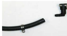
28. Secure the female quick connector included in your kit to one end of the hose using one of the enclosed hose clamps.
