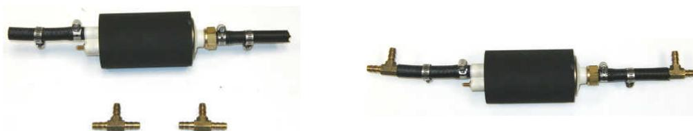
13. Using the loose second hose clamp on each of the fuel lines, secure the fuel line to the tee fitting.
