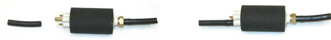
10. Using the enclosed hose clamps secure the fuel lines to the fuel pump.
