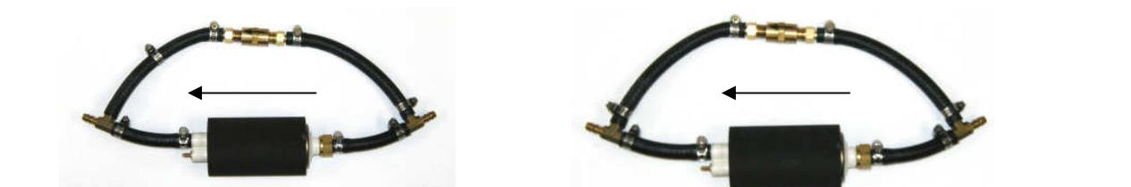
20. Find a suitable mounting location for the external fuel pump assembly. Typical location include mount the fuel pump assembly to the fuel tank shield, the inside of the frame rail, or to the bottom of the spare tire well.
