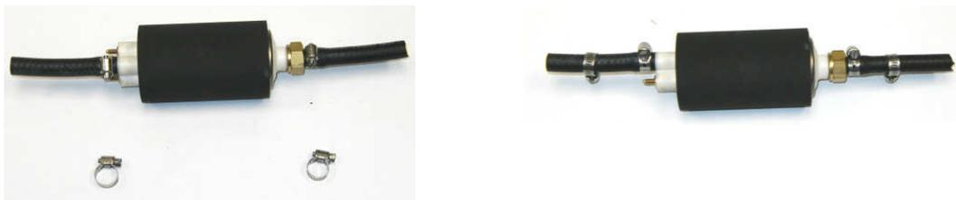
12. Insert each of the supplied tee fittings into each of the hoses coming from the fuel pump.
