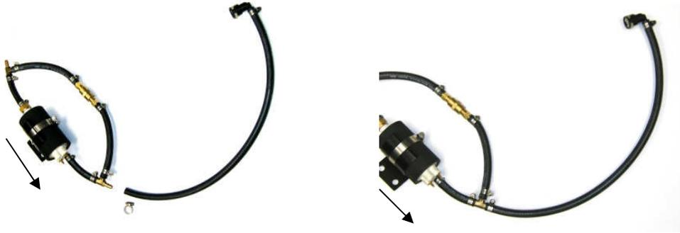
30. From the remaining section of fuel injection hose cut a length of hose, typically 20" in length, to run from the factory female quick connector removed from the filter inlet, back to the tee fitting on the inlet side of the external fuel pump assembly. You will need to install the male quick connect adapter fitting to make the connection as follows:
