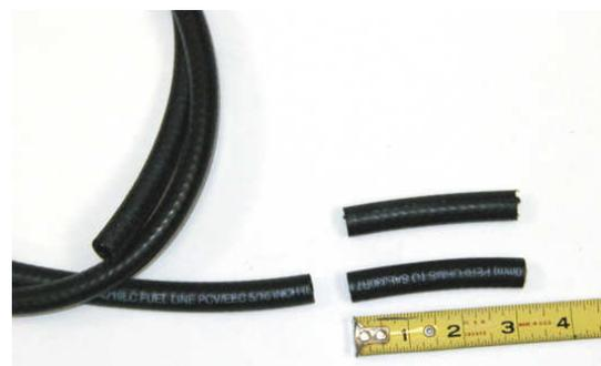
9. Slide one of the 3" lengths of hose on to the pump inlet barb and the second 3" length onto the fuel pump outlet barb.
