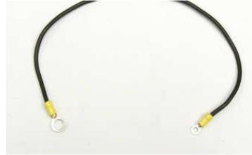
37. Using a piece of the enclosed #12 red wire, plan a route from the external fuel pump positive lead to the mounting location of the Digital FMU inside the vehicle. Cut the wire to the desired length and on one end of the wire crimp on one of the yellow #10 ring connectors to connect the external fuel pump positive terminal. On the other end of the wire crimp on one of the yellow spade connectors to connect to the Digital FMU terminal labeled "PUMP", refer to the Digital FMU wiring diagram.
