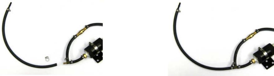
33. Connect the male quick connect adapter on the fuel pump assembly inlet to the factory female quick connect formerly attached to the fuel filter inlet.
