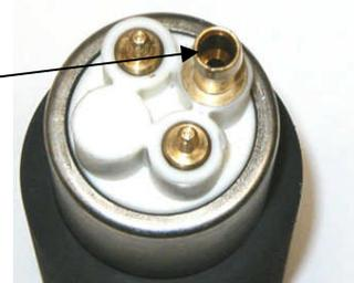
6. Apply a small amount of Teflon tape or Teflon pipe thread sealant to the 1/4" NPT threads of each of the 5/16" Barb x 1/4 -NPT fittings.
