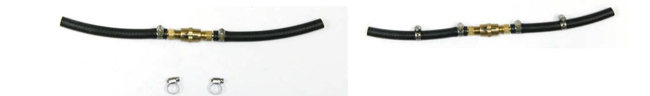
18. Insert the tee fitting on the inlet side of the fuel pump into the fuel injection hose on the inlet side of the check valve assembly and secure using the second hose clamp on the check valve hose.
