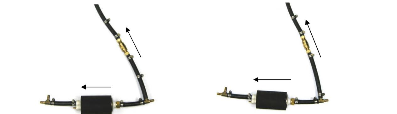
19. Insert the tee fitting on the outlet side of the fuel pump into the fuel injection hose on the outlet side of the check valve assembly and secure using the second hose clamp on the check valve hose.
