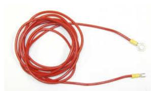
39. Mount the enclosed circuit breaker as close to the above power source as possible, cut the above #12 red wire and crimp one of the yellow #10 ring connectors on each end. Secure each of the #10 ring connectors to the circuit breaker.
