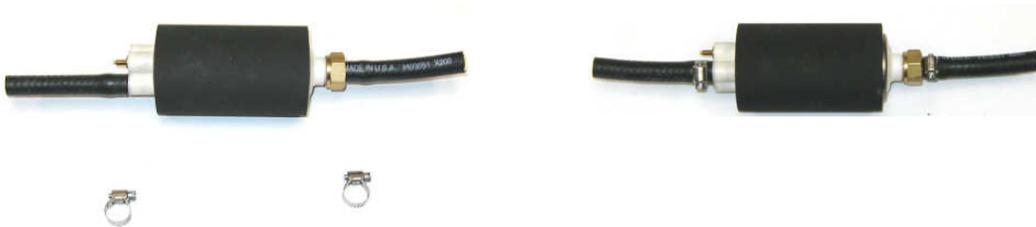
11. Slide a second hose clamp onto each of the above two lines.
