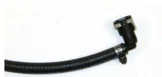
29. Using one of the enclosed hose clamps, secure the opposite end of this hose to the tee fitting on the outlet side of the external fuel pump assembly.
