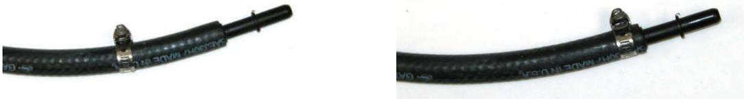
32. Secure the opposite end of the above hose to the remaining barb on the inlet side tee fitting of the fuel pump assembly using one of the enclosed hose clamps.
