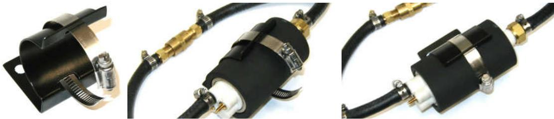
26. Remove the female quick connector from the inlet side of the factory fuel filter. You will be routing this line to the inlet of the external pump. From the external pump outlet you will then route a line back to the fuel filter inlet as follows:
