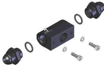
23. Remove the OEM fuel pressure sensor from the factory fuel rail and install on the Aeromotive fuel sensor adapter block, p/n 15115, using the provided screws and washers.
