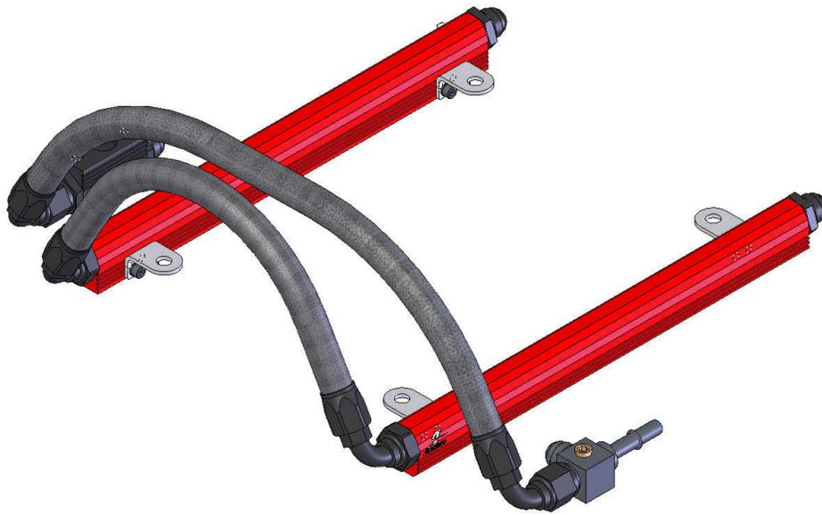
29. Connect one AN-08 90-degree hose end to the side of the fuel supply tee fitting and the AN-08 45-degree hose end to the rear of the right side fuel rail as shown below. Plan a route between the two hose ends, measure the length of fuel line needed and cut. See section titled Hose and Fitting Assembly for fuel line assembly instructions. Once the hoses are assembled, **ensure there is no debris in the hose** and install them.
