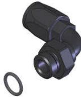
25. Connect one each of the two AN-08 90-Deg Male ORB hose ends to the front of each fuel rail. Plan a route between the two hose ends over the top of the supercharger, taking into account hood clearance, measure the lengths of fuel line needed and cut. See section titled Hose and Fitting Assembly for fuel line assembly instructions. Once the hoses are assembled, **ensure there is no debris in the hose** and install them.
