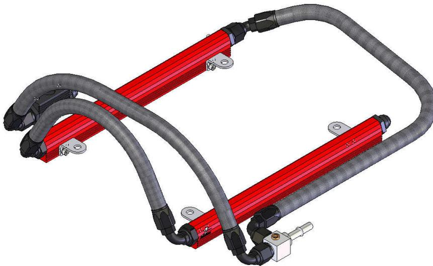
30. Connect the final AN-08 90-degree hose end to the rear of the left side fuel rail and the AN-08 straight hose end to the rear of the fuel pressure sensor block as shown below. Plan a route between the two hose ends, measure the length of fuel line needed and cut. See section titled Hose and Fitting Assembly for fuel line assembly instructions. Once the hoses are assembled, **ensure there is no debris in the hose** and install them.
