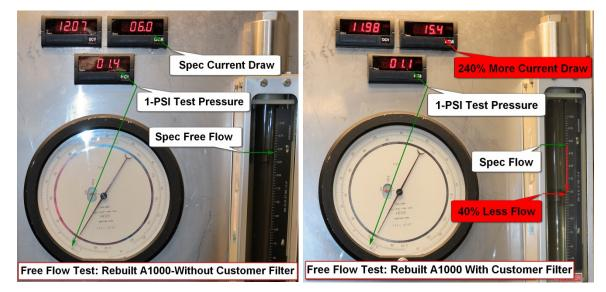
With the A1000 pump back up to snuff the customer's filter was installed after the fuel pump, just as it had been installed on the vehicle, in order to validate our theory of what the problem was. As we suspected, fuel pump performance was immediately and significantly degraded.
