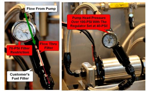
Setting the down-stream pressure up to a typical EFI level of 40 PSI brought pressure before the filter up to over 100 PSI! No wonder there was damage. Lessons learned? A.) Install a genuine Aeromotive fuel filter after the fuel pump (See Tech Bulletin #102). B.) Monitor filter condition, especially in new systems, to ensure the element is clean and free flowing, thus preventing drivability problems and protecting instead of harming the pump.
