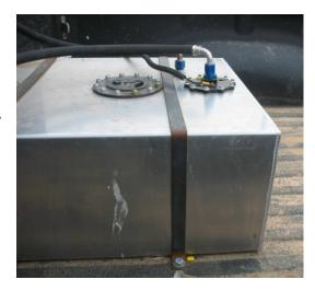
With the Stealth Fuel Cell involved, we knew the root causes of most drivability problems were in fact eliminated, namely incorrect fuel tank baffling and inlet restrictions resulting from an undersized feed line and/or improper inlet filtration (see Aeromotive Tech Bulletin #802 and #101 respectively). It was clear that the source of the problem was located elsewhere in the system.
