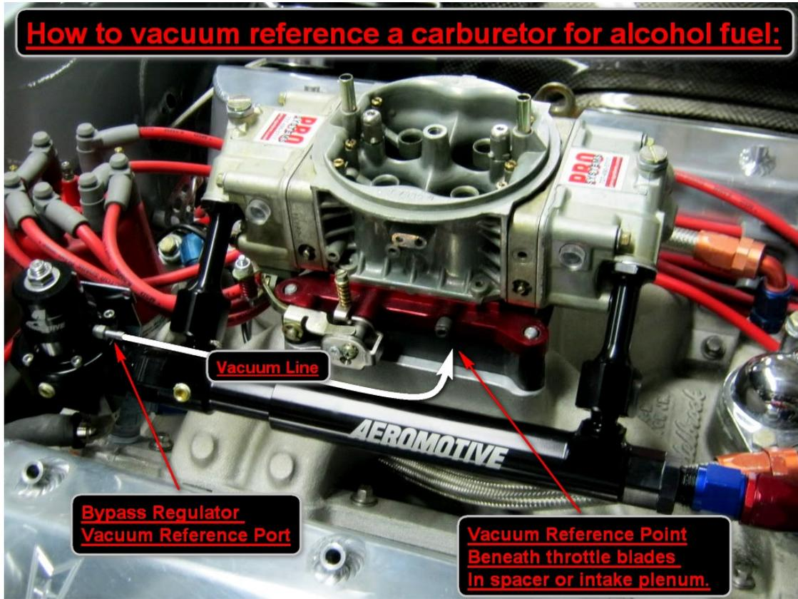
Taking advantage of vacuum/boost reference capability on a naturally aspirated, alcohol engine, fuel pressure can be set higher for WOT operation but reduced at idle, using the vacuum in the intake. Although we can't completely control idle and WOT fuel pressure with vacuum like we can with an Aeromotive Belt Drive Pump and Double Adjustable Regulator, a real difference in pressure from idle to WOT is possible, and every little bit helps when it comes to alcohol carburetion.
