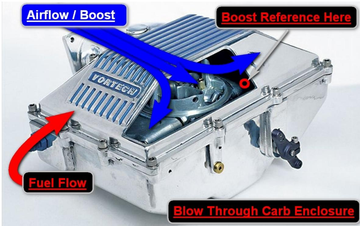
Note: Using a bypass regulator creates a dynamic fuel delivery system that has benefits for all carbureted engines, naturally aspirated, draw through supercharged, nitrous, etc. So do not hesitate to use a bypass regulator for any carbureted engine application, see TB-801 for more info. However, for carbureted engines that do not require a boost reference, like roots blown and nitrous combo's, the regulator's vacuum/boost reference port should be left open to atmosphere, never plugged.
