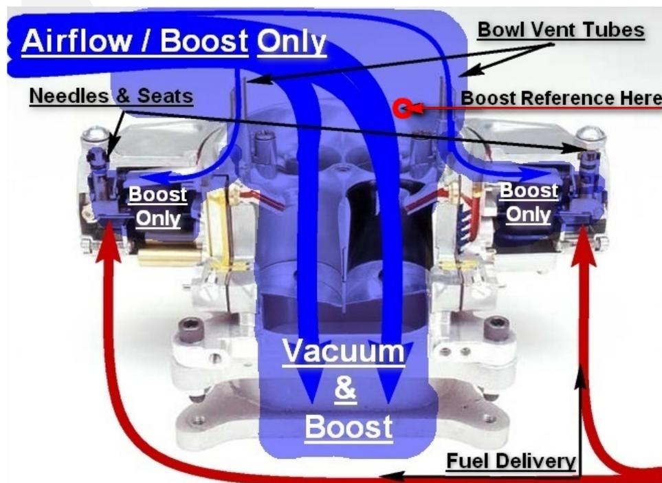
The boost reference line on a blow through engine should reference positive pressure only (that is boost), not vacuum, and be connected to the carburetor box or hat rather than the intake manifold. Does a blow through carburetor in a "box" or enclosure require boost reference? The benefits of enclosing a blow through carburetor do not include avoiding use of a boost referenced fuel system. Always boost reference blow through carbureted engines, regardless of using a box or hat.
