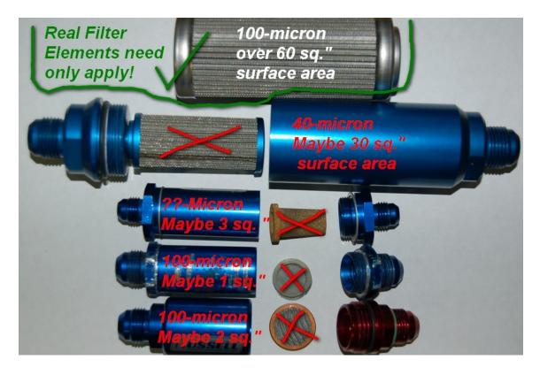
Above are various versions of "100-micron" fuel filters/elements. Note: the top element is the Aeromotive 100-micron element P/N #12604, as found the fuel filter assembly P/N #12304. Note the various filters all have "billet" housing, with AN connections, and can be disassembled for inspection and cleaning. Also, note that all are sold and recommended as appropriate pre-filters.
